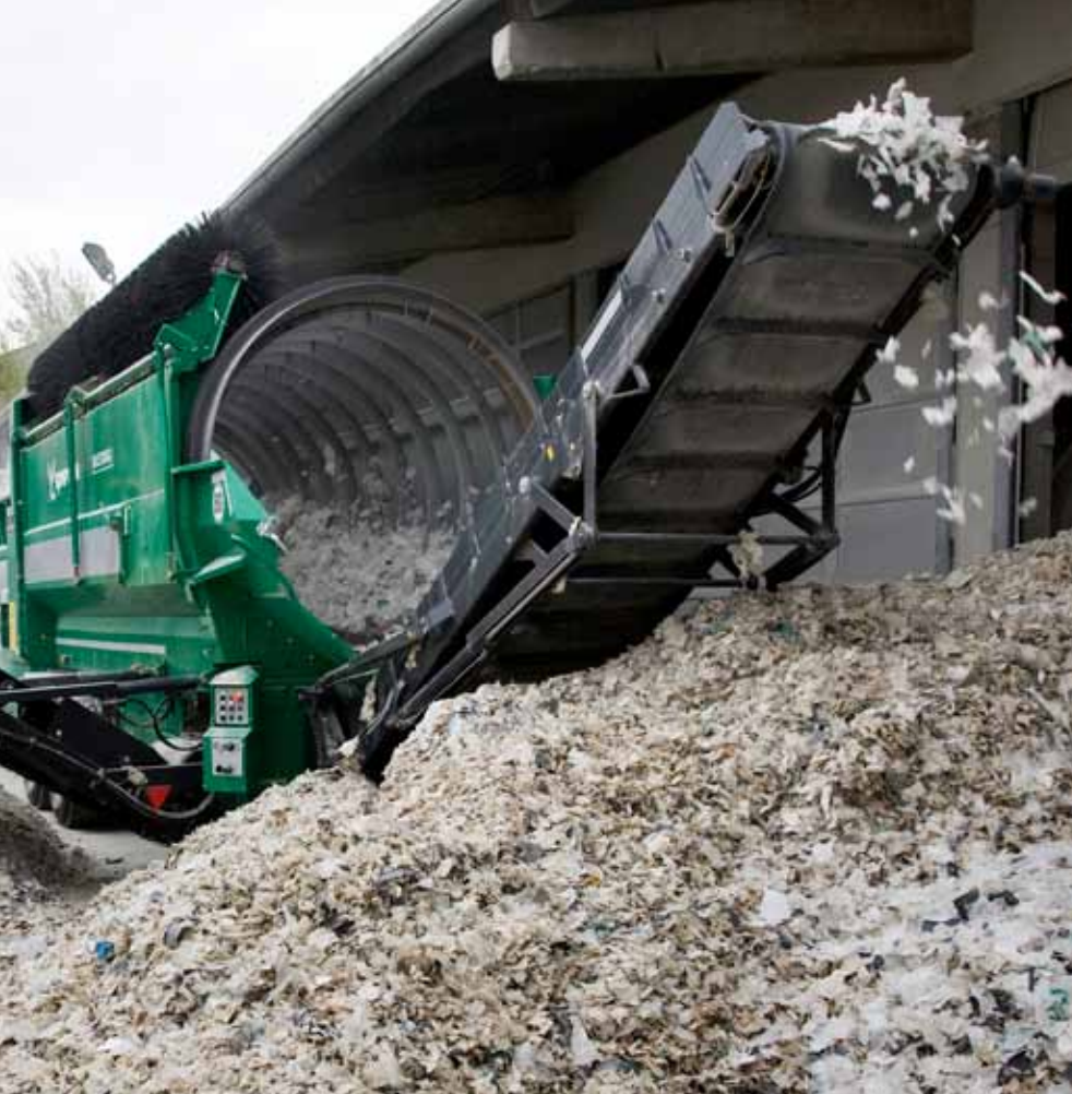
A Mustang drum screen screening shredded safety glass film.
