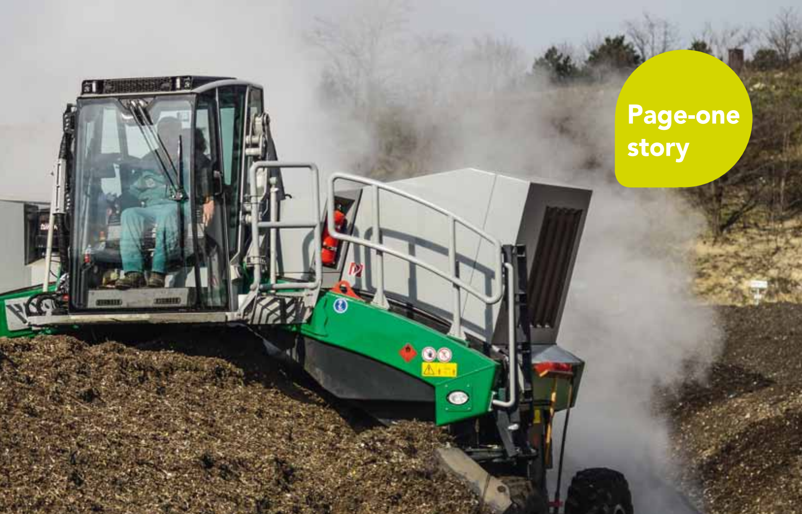
Stress test for the new Topturn X55: Even with heavy material, Stefan Wieder goes through considerably more than 1000 cubic metres per hour.
