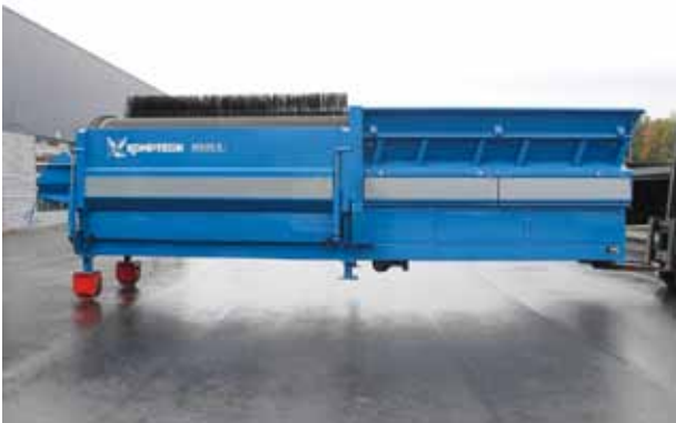
Mobile trommel screen in stationary application
